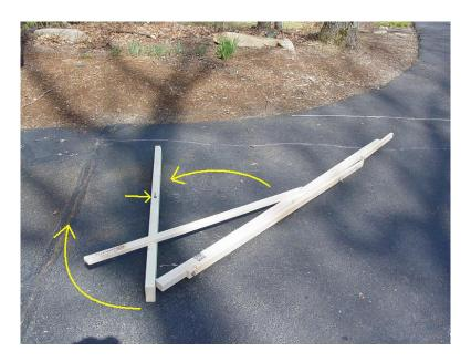
3. Attach the support arm to the bolt, using a single nut and washer. The stand is designed that any nut which is removed to assemble or disassemble the stand is single; any location where the nuts are not to be removed will have double nuts. You will need a 7/16" wrench to tighten the nuts; this is the only tool required.
