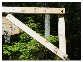
7. Attach the free end of the lower crossbar to the bottom bolt on the right side of the stand.
