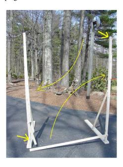
5. Detach either diagonal brace (D5 or D6) from the 2 x 4 base plate. Swing the brace in **FRONT** of the 5" bolt so the brace can pivot forward flush with the upright, and 2 x 4 can hinge flat against the upright.
