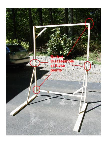
2. Remove the single nut from the attached end of the small diagonal front brace from the lower crossbar (D1). Reattach the nut and washer to the bolt to "store" them. Repeat for the crossbar itself (D2).
