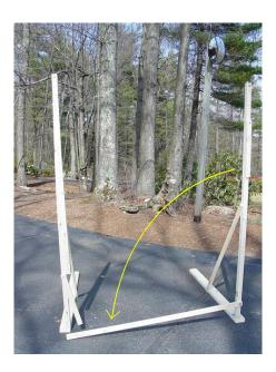
6. Attach the free end of the upper crossbar to the top bolts on the left side of the stand.
