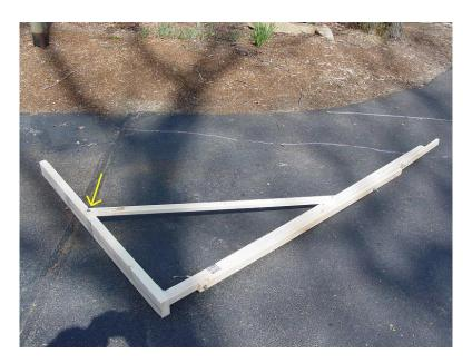
4. All assembly/disassembly points on the units are labeled with A#/D#. These are the assembly/disassembly order numbers. For example, **A1/D6** means assemble the unit starting at this point (A1) and disassemble at this point last (D6).
