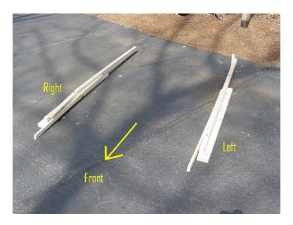
2. Unfold the 2 x 4 from the upright, and swing the diagonal support arm back toward the 5" bolt in the middle of the 2 x 4.
