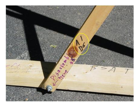
5. Repeat the process of attaching the diagonal support arm from the upright to the 2 x 4 for the other half of the stand. Set the two halves upright approximately 5 feet apart.
